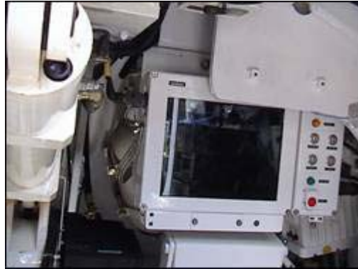
Figure 10: The location of GDU in the howitzer.
